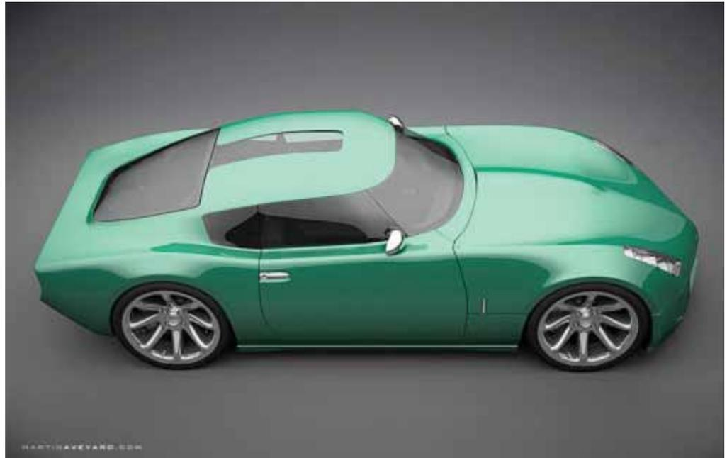
Triumph purists will be pleased to know that the one-piece front-end/bonnet is still evident and conceals a straight-six engine, albeit with increased power and capacity. The power bulge and air vents on top of the bonnet are design cues that have also been carried over from the original. The vents have been simplified aesthetically, but as chrome decor pieces they are now a more prominent feature.
