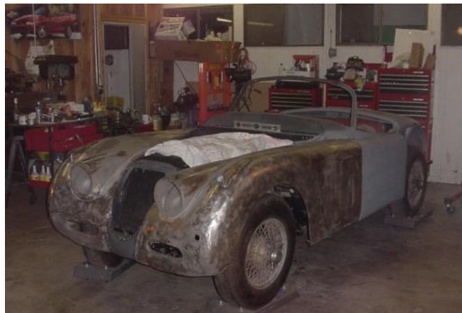
Wings welded in place
