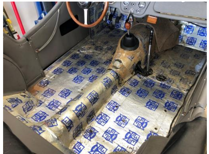
2 Old Carpet & Underfelt Removed
