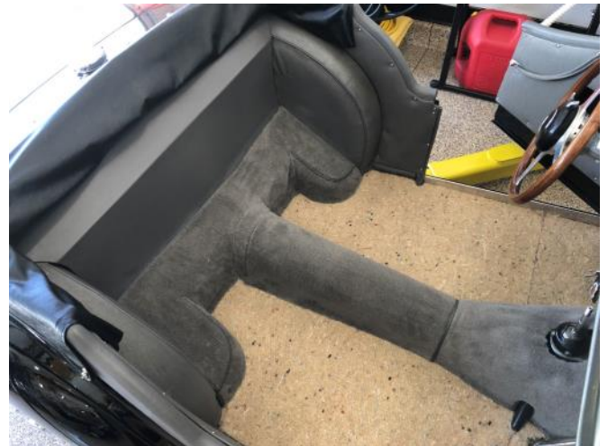
4 Tunnel and rear carpet installed
