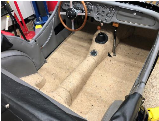
3 New underfelt installed
