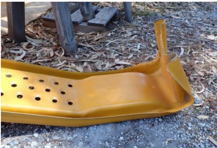
Bent ramp (upside down to show damage)
