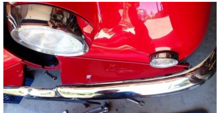
Damaged paint by the bumper
