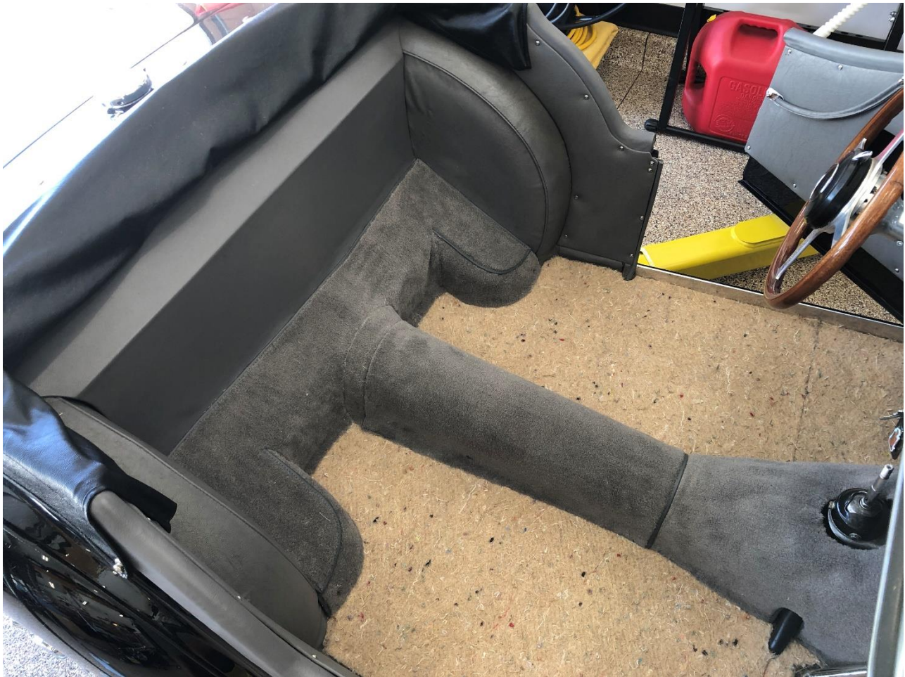
Figure 4: Tunnel & rear carpet installed
