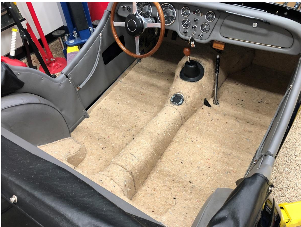
Figure 3: Jute underfelt installed
