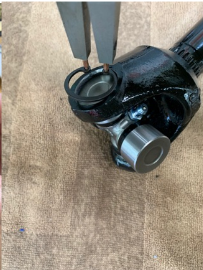
Install snap ring on one side.
