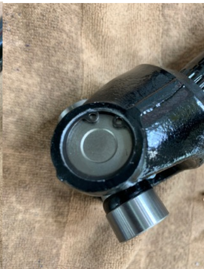
Install snap ring on other side
