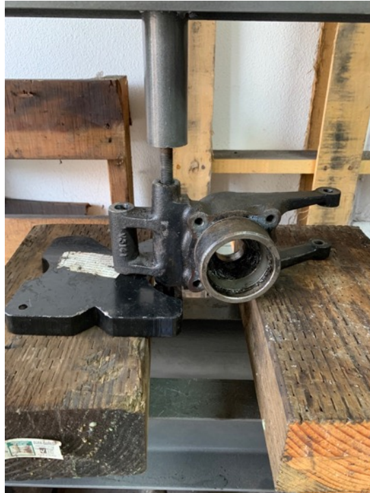
Pressing radius rod bracket bolt out
