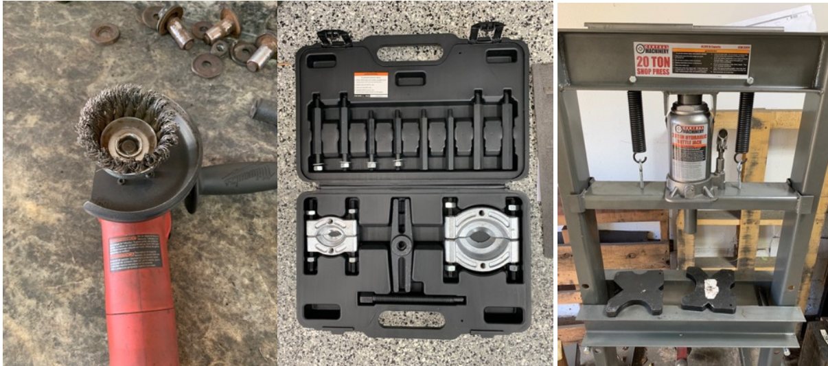
Angle grinder with wire & cutoff wheels, Universal bearing puller, 20 ton press
