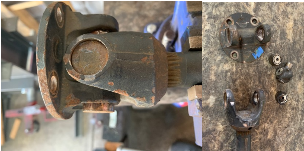
Exposed bearing cup to pull off, cutting wheel destructive method
