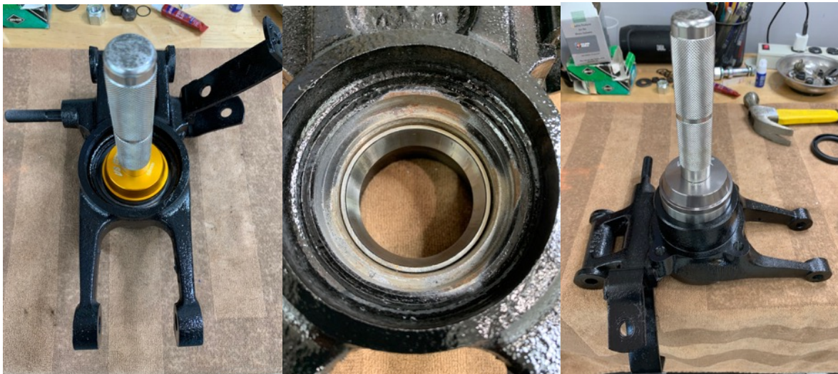
Inner race and driver, inner race seated, outer race ready for driving in
