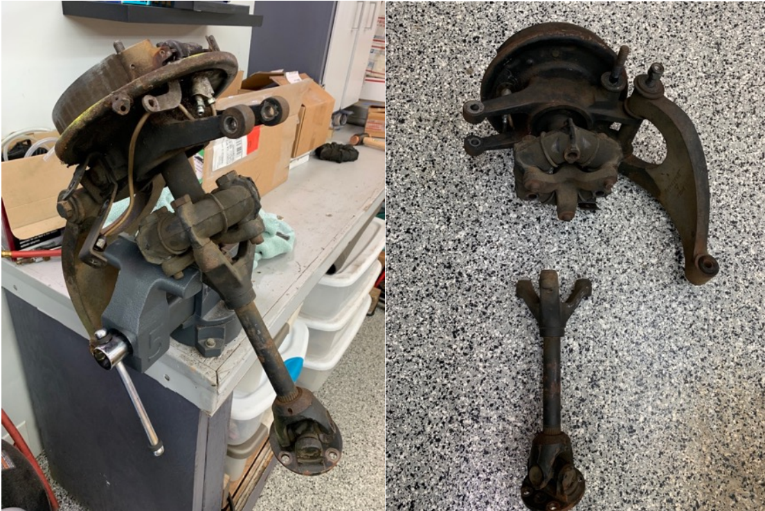
Assembly in vice, inner axle separated
