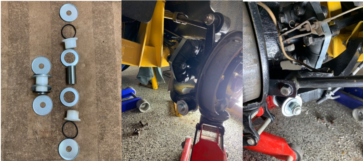
Trunnion bushings and seals, wishbone attached, radius arm attached
