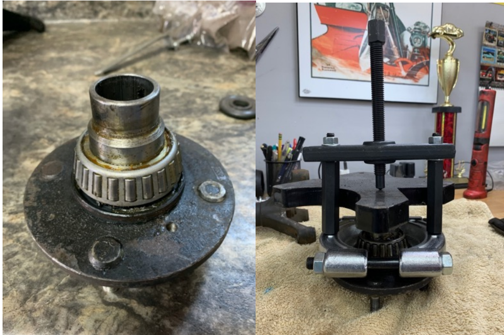
Hub and outer bearing, Puller assembled for removal
