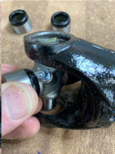
Install snap ring on one side.
