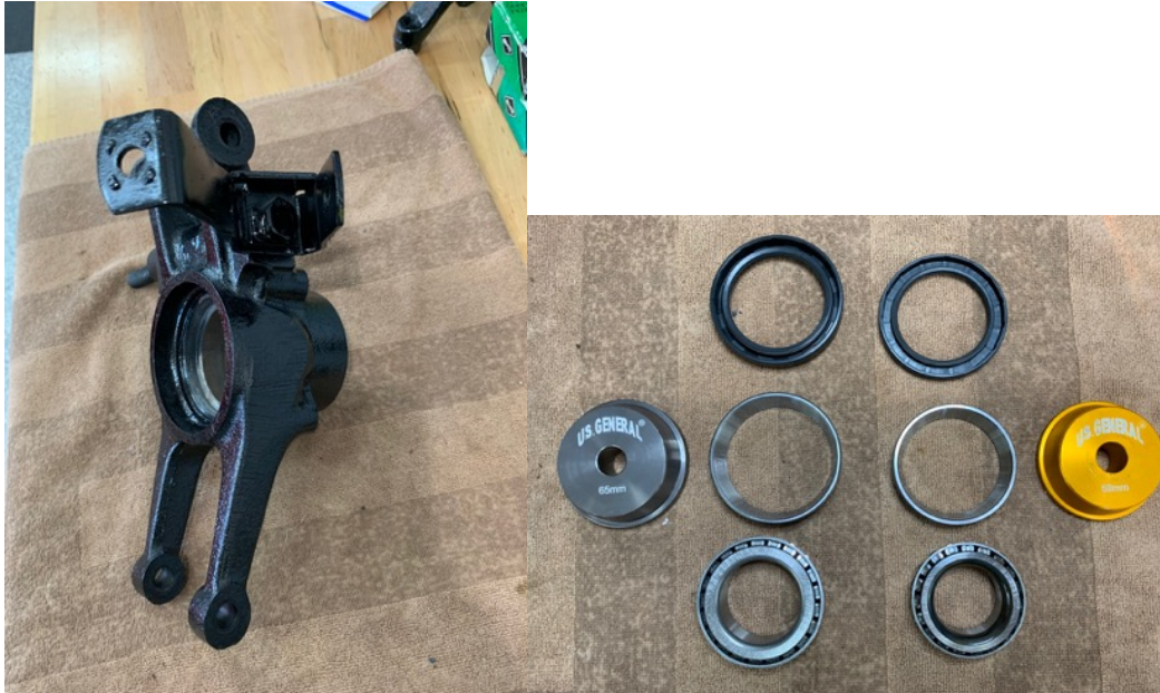
Inner race and driver, inner race seated, outer race ready for driving in
