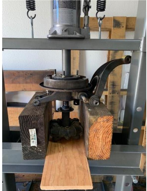
The object of my desire is getting smaller and easier to handle, wishbone is still painfully intrusive. I flip everything over so I can extrude the hub. The easier removal of the axle from the hub gives me hope the hub will be just as kind. I am rewarded with a smooth extraction and the corresponding bang as it lands on my improvised catch shelf.
