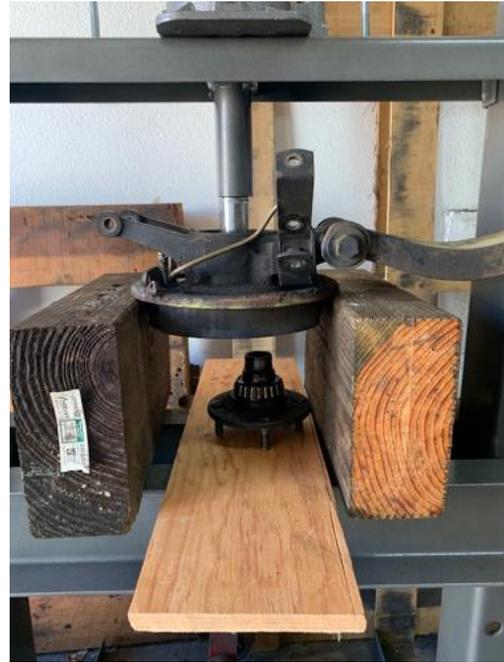
The brake backing plate is now four easy bolts away from freedom and a major dimensional object dislodged. The assembly is getting smaller and easier to deal with, despite that pesky wishbone.
