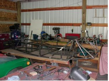
I then rebuilt the motor and trans from the donor car for the Clone Lotus Seven so I could start to fit them and make adjustments to the frame as needed, as the MGB engine is larger than the original Lotus Seven America had when they were
