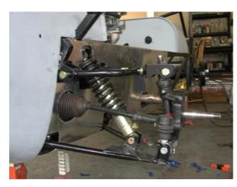
It seemed that I would get an assembly installed like the upper and lower a-arm and then find out that I could not get the skin installed with the a-arms in place and would have to remove those assemblies and start over. One good thing about having to do that was I knew that every part fit and would work so in the end it made the car much better. I knew everything fit and worked. At this point I had a basic car that would start and run and stop but still needed to be finished.
