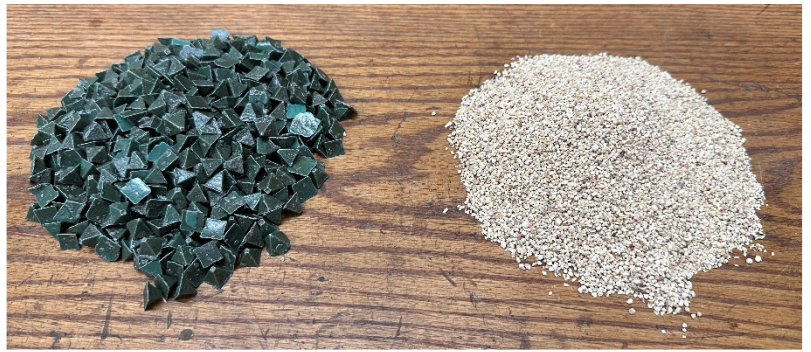
Figure 5: Harbor Freight tumblers and both types of media – resin and corn
