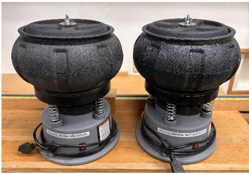
Figure 5: Harbor Freight tumblers and both types of media – resin and corn
