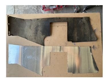
The small end of the valence is bent in two places to wrap around the front of the engine and mount to the radiator. Laying the original as a template on top of the flat new valance, I marked the top and bottom of the aluminum to identify the crease line. Using a short piece of 2x4, I lined the edge up with my marks. While placing a hand on the 2x4 to stabilize it I slowly lifted the aluminum to match the angle of the old valance template.
