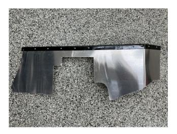
Test fitting revealed that larger cutouts around the suspension were required for clearance as the old soft material valance was more flexible for installation and rested on chassis parts. I didn't want to introduce metallic vibrations nor wear the paint off of the chassis, so I cut a larger space in the valance for the suspension. In the end it was an enjoyable, easy project and looks really nice under the bonnet.
