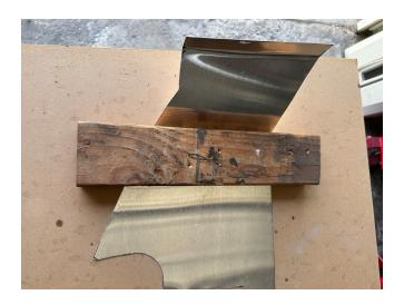
Once this was done, the new aluminum valance was placed into the refurbished support bracket, a marker was used to translate the old rivet holes onto the aluminum and then drilled out. I then mounted the aluminum to the bracket with #8 screws, lock washers and nuts.
