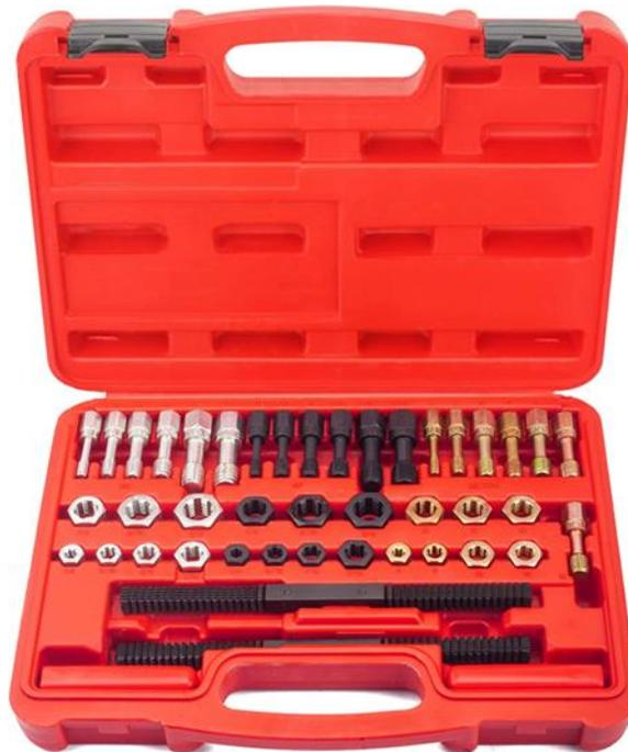
Figure 4: Thread restorer kit
