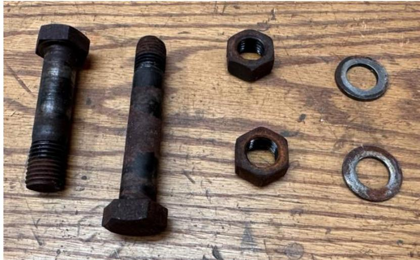
Figure 3: Parts after ultrasonic cleaning
