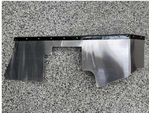
Test fitting revealed that larger cutouts around the suspension were required for clearance as the old soft material valance was more flexible for installation and rested on chassis parts. I didn't want to introduce metallic vibrations nor wear the paint off of the chassis, so I cut a larger space in the valance for the sus-
