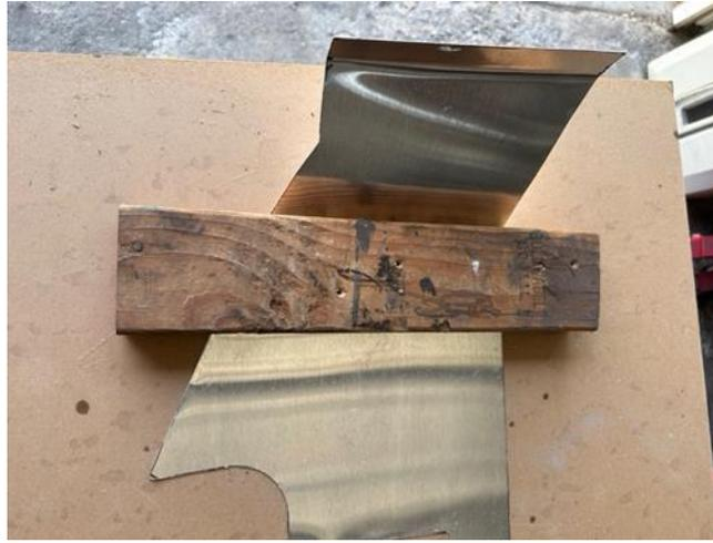
Once this was done, the new aluminum valance was placed into the refurbished support bracket, a marker was used to translate the old rivet holes onto the aluminum and then drilled out. I then mounted the aluminum to the bracket with #8 screws, lock washers and nuts.
