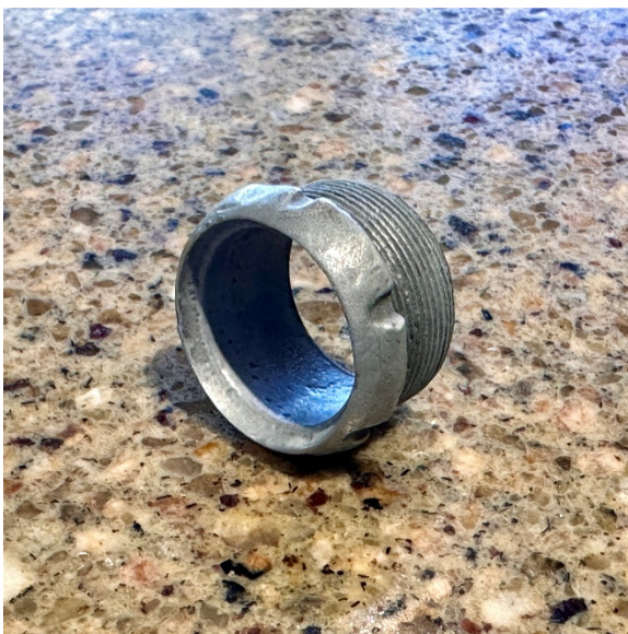
The bezel after 60 seconds in Metal Prep (no sanding yet)
