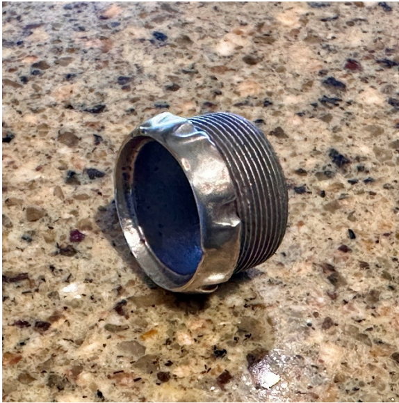
The bezel after nickel plating and steel wool polishing
