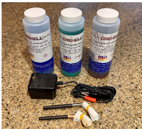
Flash Copper, Nickel and Copy Chrome solutions, 2 wands with bandages and the power supply
