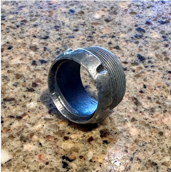
The bezel after media blasting and wire wheel cleanup (no sanding yet)
