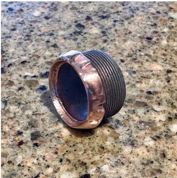
The bezel after Flash Copper plating AND sanding and steel wool polishing
