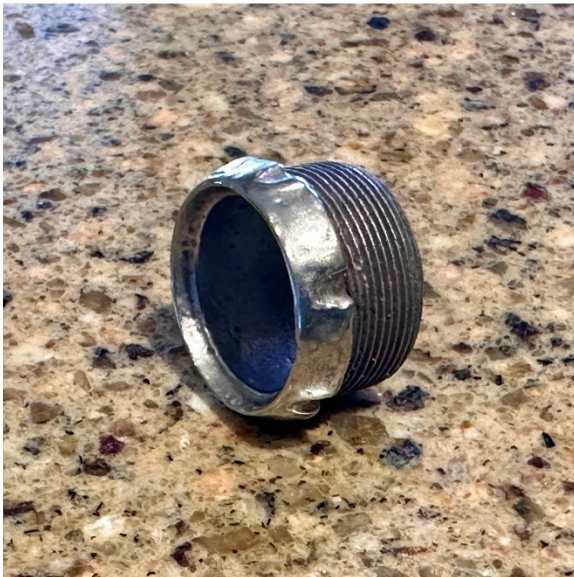
The bezel after Copy Chrome and steel wool polishing
